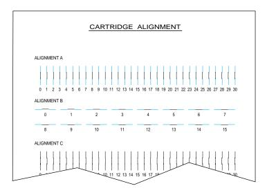
From each group on the test page, locate the number under the alignment pattern that comes closest to forming a perfectly straight line.
